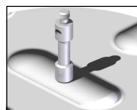
These are used for probing holes in thin sheet material. In addition, various threaded features can be probed and the centers of tapped holes located. Ball-ended cylinder styli allow full datuming and probing in X, Y and Z directions, thus allowing surface inspection to be performed.
